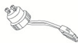
PSA31 GU10 to Ideal connector PSA31 Available for retrofitting GU10 housings (Not shown above)
